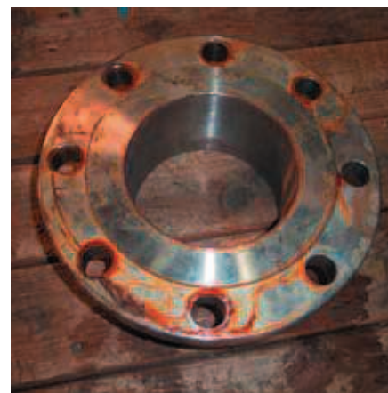
Fig. 5. RVS 304 flange contaminated by ferruginous water.
