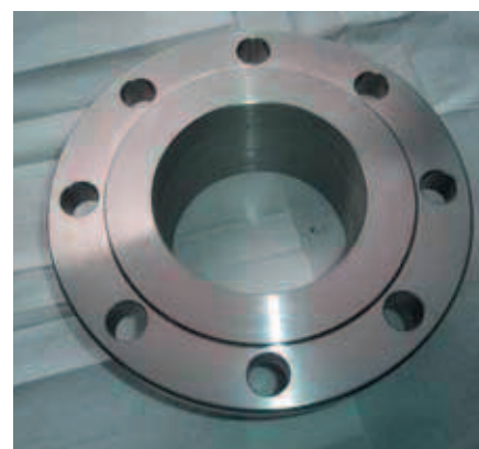
Fig. 6. The same flange as in Figure 5 but cleaned with Innosoft B570 and coated with a nanolayer.
